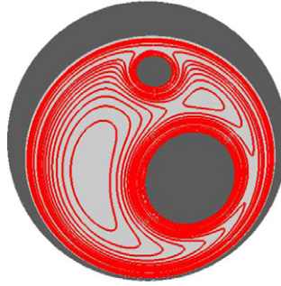
Fig. 2. Point vortex trajectories in a basin with two islands.
